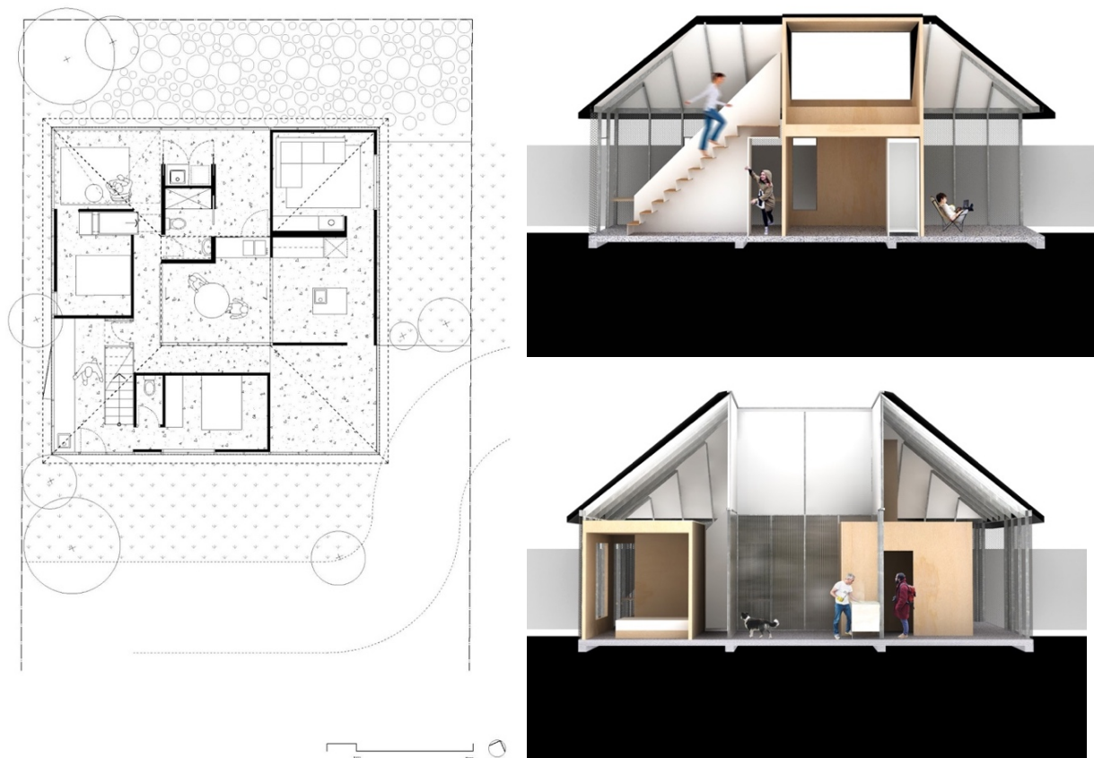
Figure 2. Pavilion House , Jacqui Alexander. Floor plan demonstrates the home reconceptualised as a series of atomised rooms. Interior sectional perspective renders show furniture elements that mediate the relationship between household occupants, enabling more or less space to be rented out on-demand.
