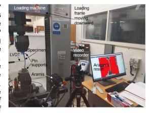
GFRP laminates on their failure modes and capacity.
