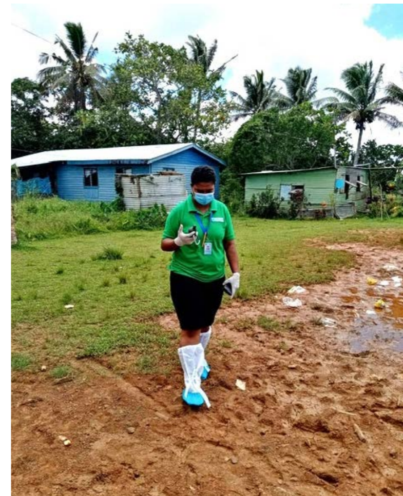
Community Fieldworker Meiva Setoka conducts surface-soil sampling with bootsocks in a settlement in Suva, Fiji.
