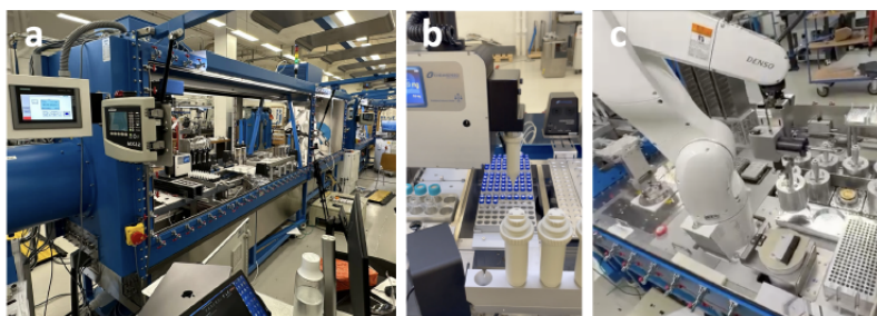
Figure 1. ACAP Energy Materials Platform, located at the MCN. (a) Front view of the multi-glovebox system hosting the platform, (b) Formulation capability, including gravimetric solid dispensing tool, (c) Film formation capability.
