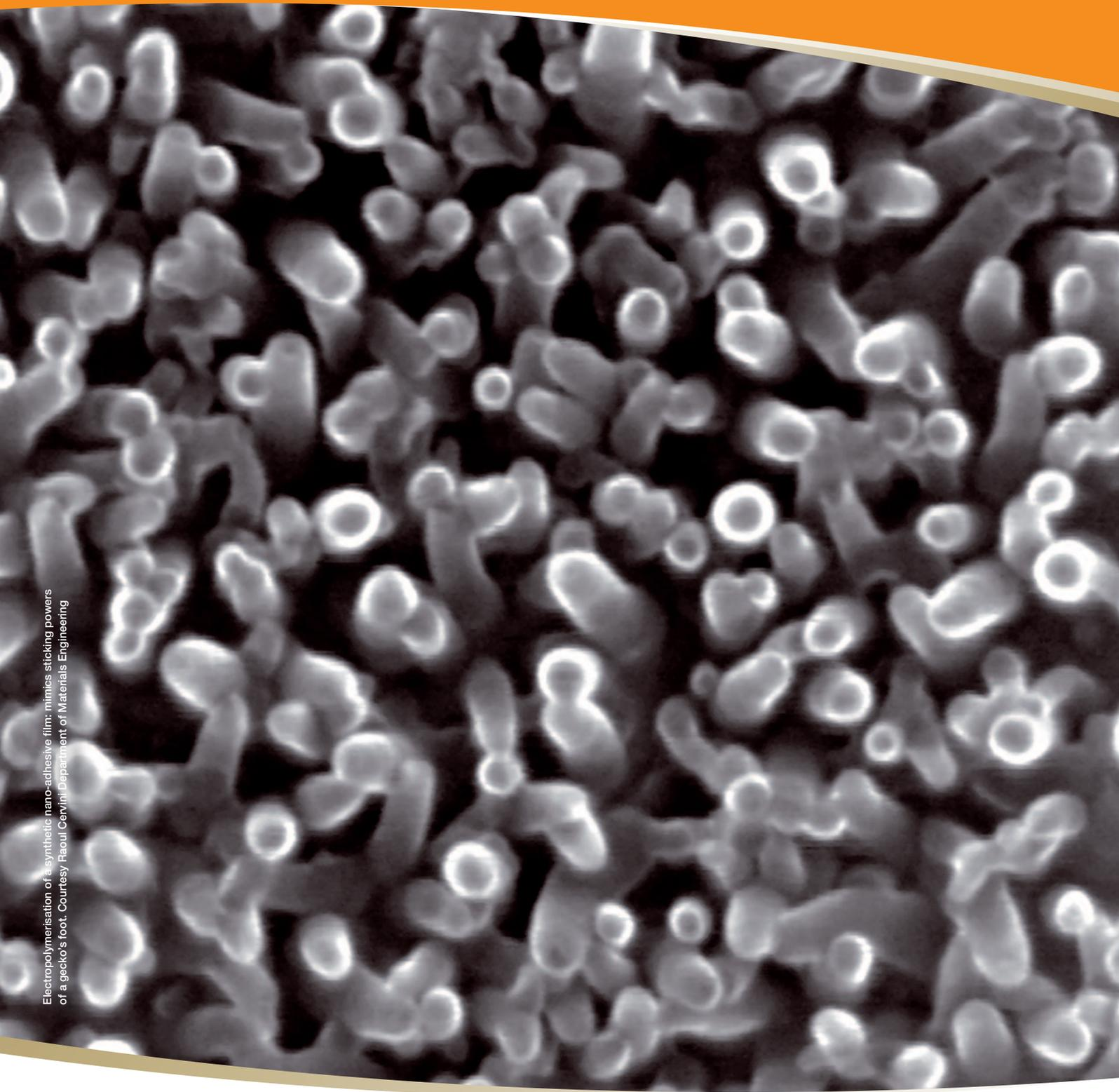
Electropolymerisation of a synthetic nano-adhesive film: mimics sticking powers of a gecko's foot. Courtesy Raoul Cervini/ Department of Materials Engineering
