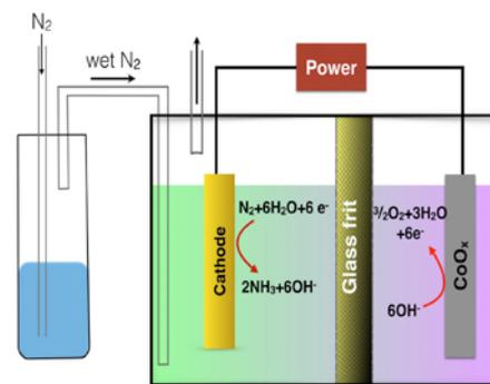
Figure 1: Schematic of a typical electrochemical cell for N<sub>2</sub> reduction.
