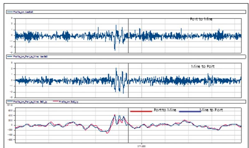
**Fig 6. There is a clear correlation between weld shape and the corresponding vehicle dynamics.**
