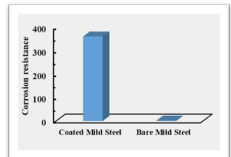
Figure 1. Corrosion resistance of graphene-coated vs. uncoated mild steel.
