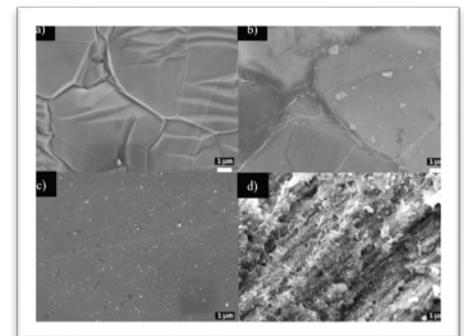
Figure 2. SEM results for (1) graphene-coated and (2) uncoated mild steel following 1008 hours of immersion in an aggressive salt solution.
