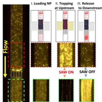
The collected high-concentration batch can be released 'on-demand' by turning off the ultrasound activation and diverting to a collection reservoir.
