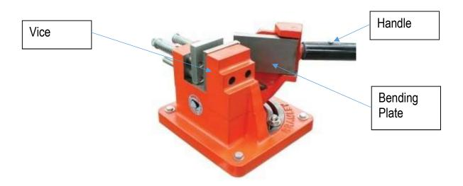
This manual bender is used to cold bend steel and other metals to angles between 0 and 90 degrees. It is capable of bending mild steel flat bar to a size of 100 x 8mm or 50 x 12mm and round bar to approximately 25mm in diameter. If unsure of its capabilities, always check with a technician prior to use. Be aware that it may bend the material but damage the structural integrity of the metal at the bend, especially with softer metals such as aluminium.
