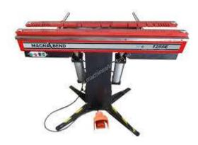
This machine is used for bending sheet metal up to 1.6mm in thickness and uses a powerful electromagnet to clamp down the sheet for bending. It is quick to use and versatile for making objects and shapes with multiple bends such as boxes.
