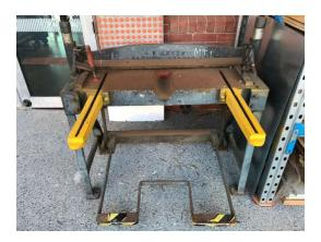
The guillotine is used for cutting medium to large pieces of sheet metal. It is ideal for cutting straight edges and can cut a maximum sheet width of 900mm.
