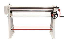
The sheet roller is a useful machine for creating curves and rolls in sheet metal material and also some wire.
