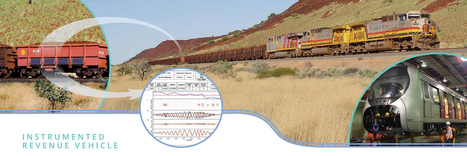
The Instrumented Revenue Vehicle (IRV) program commenced in 2001 and has since provided innovative strategies for condition monitoring and targeted condition or evidence based economical track maintenance planning. The data recorded on these vehicles is also used for developing appropriate driving strategies and assessing rollingstock performance.
