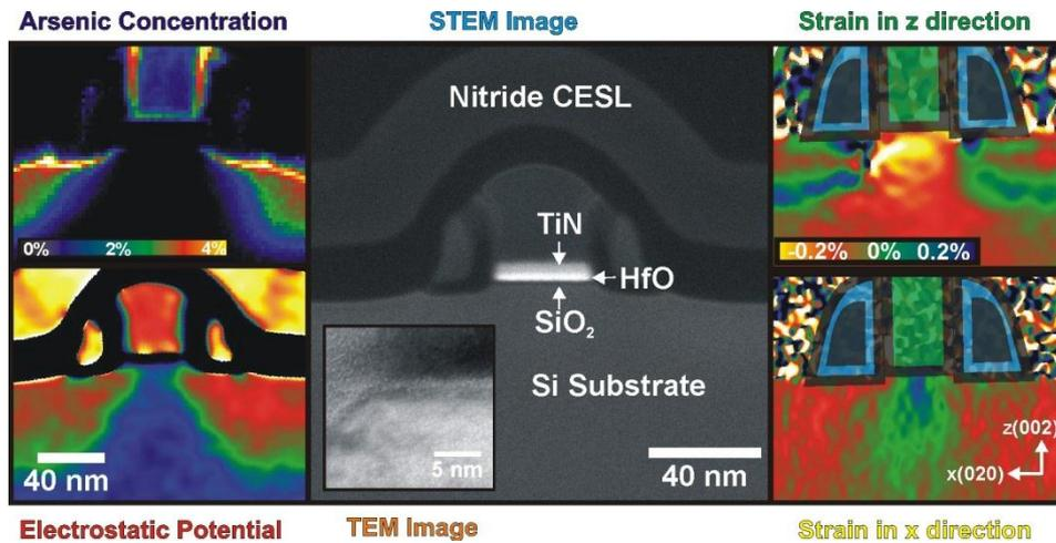
Figure 1: shows an arsenic chemical map acquired by EELS, a STEM image, strain maps acquired by dark field electron holography and a map of the electrostatic potential that has been acquired from the same TEM specimen.
