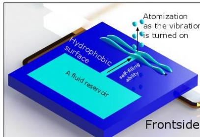
Figure 2 Atomisation occurs as the vibration is turned on.
