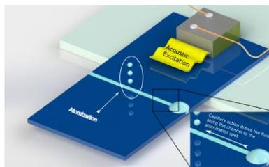
Figure 1. Capillary action draws fluid into the channel.
