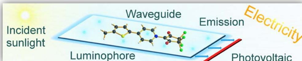
Figure 1. Graphical representation of a typical LSC
