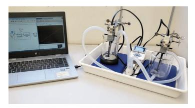
Lego Lab Live - the new online, kit-based lab for CHE3162 uses Lego Mindstorms components. Students will be able to remotely access, configure and run the apparatus themselves, generating their own data and enhancing their learning experience
