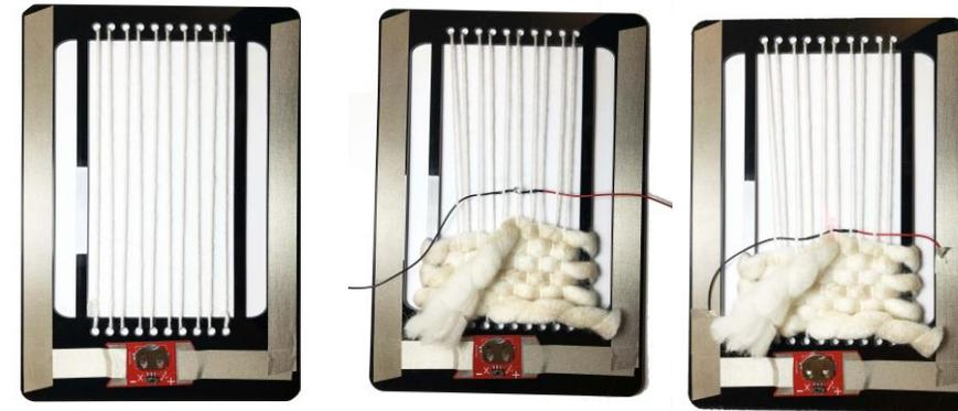
1. Tape battery holder to weaving loom with silver conductive tape. Tape across the bottom and up the sides – not across the top. The positive and negative sides must be separate.
