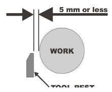
Set the height of the tool rest so that the cutting edge of the chisel is exactly in-line with the centerline.
