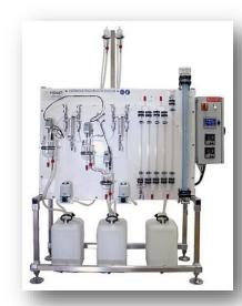
ular reactor. The reactors facilitate experiments like the dispersion of NaCl in water for residence time determination and the saponification of ethyl acetate by soda, offering practical insights into chemical reaction dynamics.
