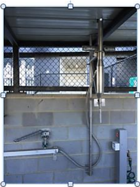
Fig. 3. Gravity fed dewar and spring return handle.
