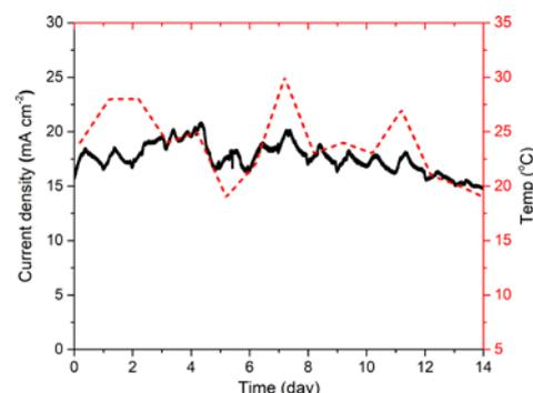
Figure 4. A 14-day stability test of our electrode in neutral media plotted together with temperature variation during the test period.
