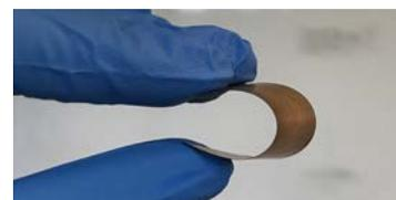
Figure 2. Photograph showing the mechanical stability of our electrode.
