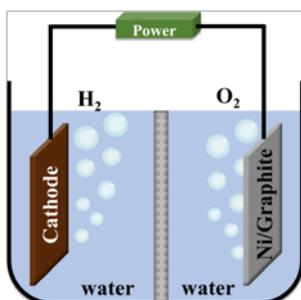
Figure 1. Illustration of a typical electrochemical cell for H<sub>2</sub> production.
