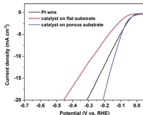
Figure 3. Linear scan voltammeteries obtained on Pt wire and our catalysts in neutral phosphate buffer.
