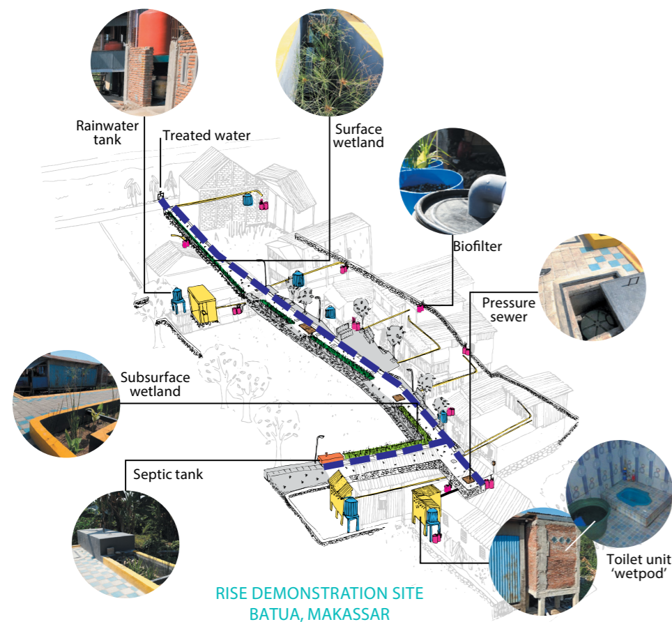
The elements of the RISE approach, implemented at the Batua demonstration project in Makassar, Indonesia
