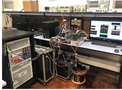
Figure 23: The experimental setup used for validating the performance of the feedback linearization compensator.
