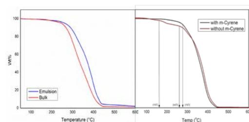
Figure 2. Thermal stability of m-Cyrene homopolymers (left) and coatings with and without m-Cyrene (right).
