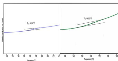
Figure 1. Glass transition temperature of m-Cyrene homopolymer by emulsion polymerization (left) and bulk polymerization (right).
