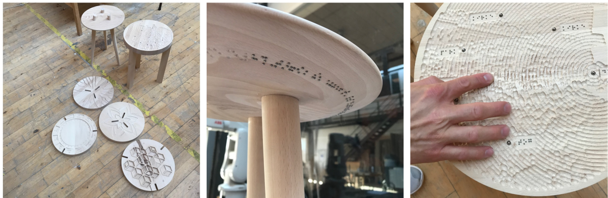
Figure 14. Accessible variations for designers within project and script framework, for unique prototypes fabrication achievable through advanced CNC manufacturing and robotic fabrication (left). Braille was inserted as extended information on underside (mid), and prominently on display within stool surface illustrating city diagram (right).
