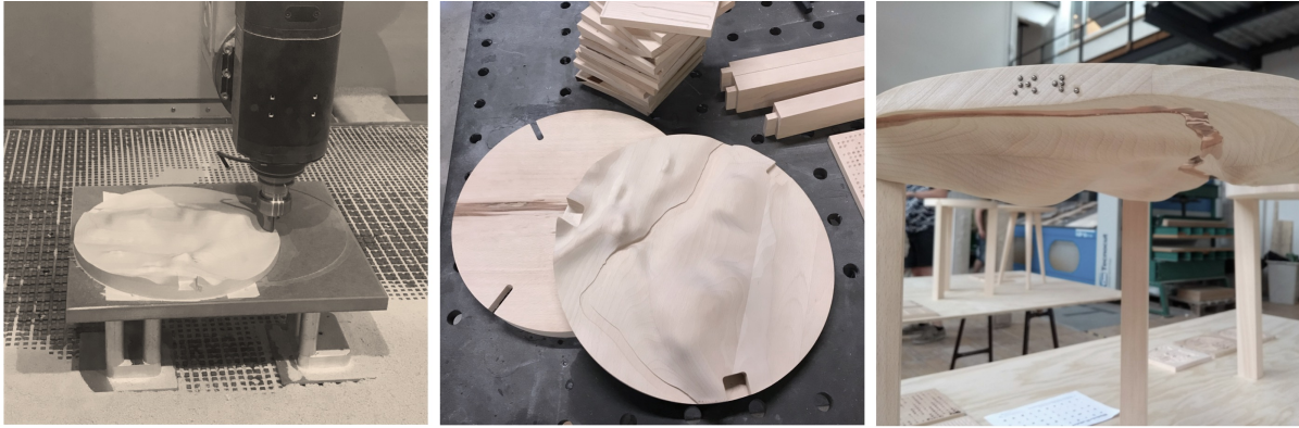
Figure 11. Multiple Tooling processes from routing deep topography in stool surface through 5axis CNCing, robotic milling and manually embedding Braille.
