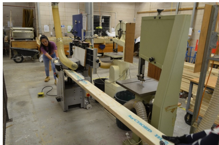
Students using thicknesser-planer to reduce LVL expansion.
