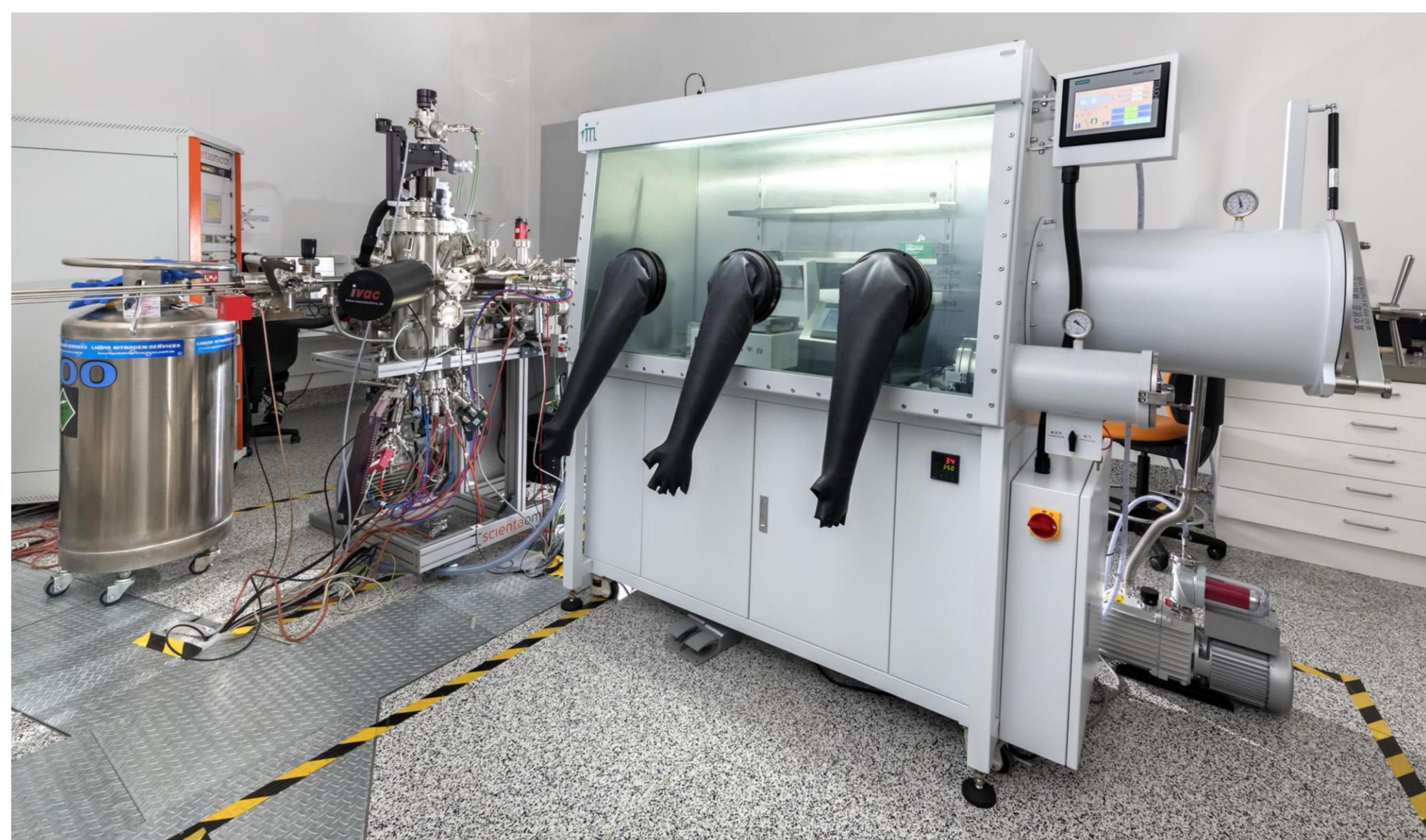
Combined MBE-Glovebox-UHV Suitcase system in our lab.
