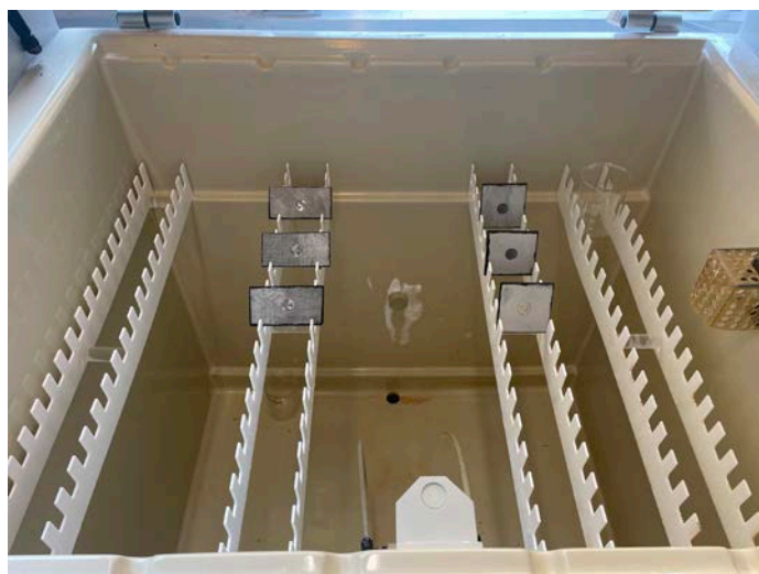
Salt spray test chamber with cold spray and thermal spray specimens. The test was performed according to ASTM standards to evaluate the atmospheric corrosion in marine-like environment
