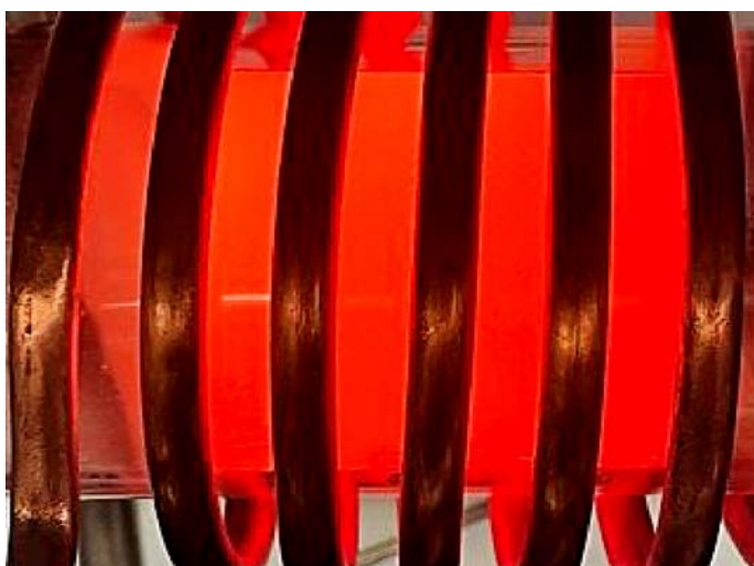
Inductively heated monolith at 900°C
