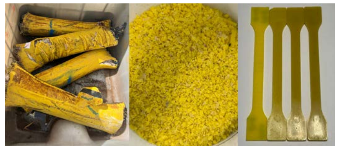
(L-R) Flowlines cut down to 1m size, followed by shredding of the outer sheath (outer layer) followed by injection moulding into new products
