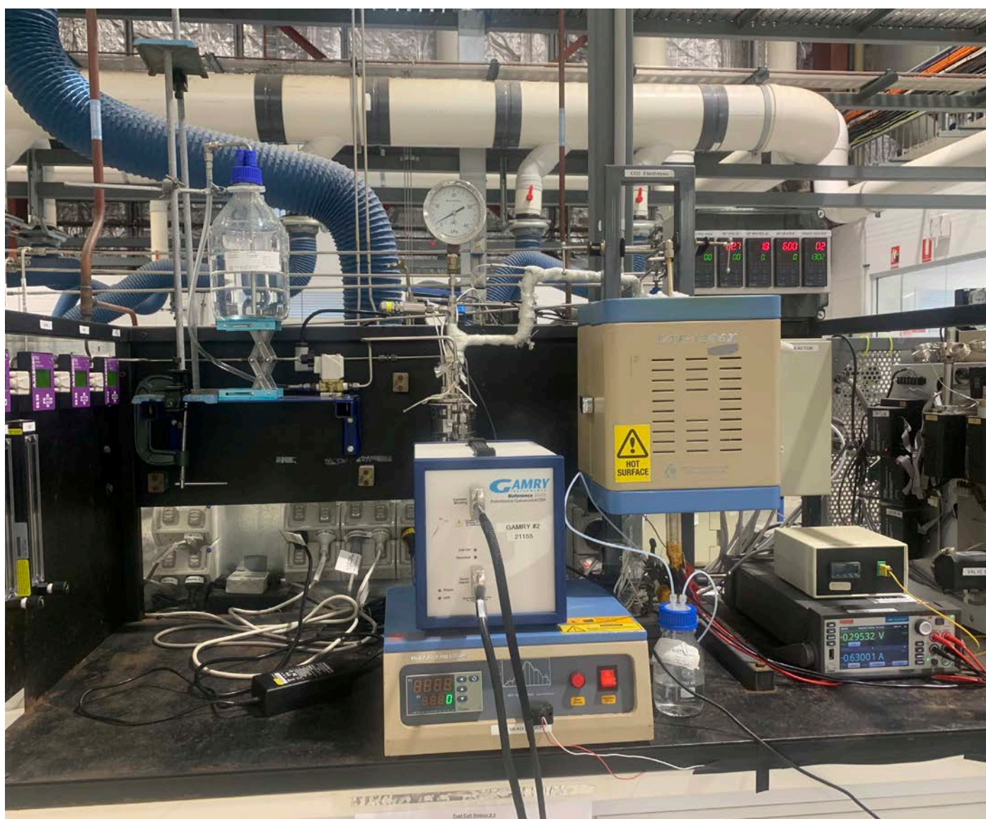
High-temperature CO 2 electrolysis setup for catalyst and electrode evaluation (Curtin)
