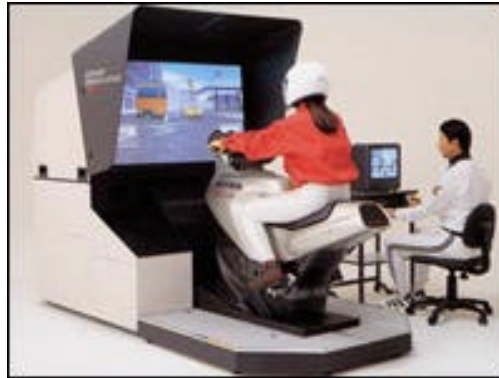
Figure 8.1 The first generation Honda motorcycle riding simulator. Image from http://www.ssdcl.com.sg/simulatorlhonda_motorcycle.asp
