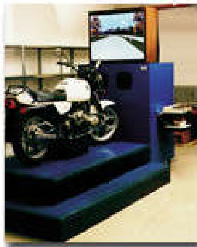
Figure 8.4 The motorcycle simulator developed by Dr-Ing Reiner Foerst GmbH. Image from http://www.drfoerst.de/e_n8m.htm
