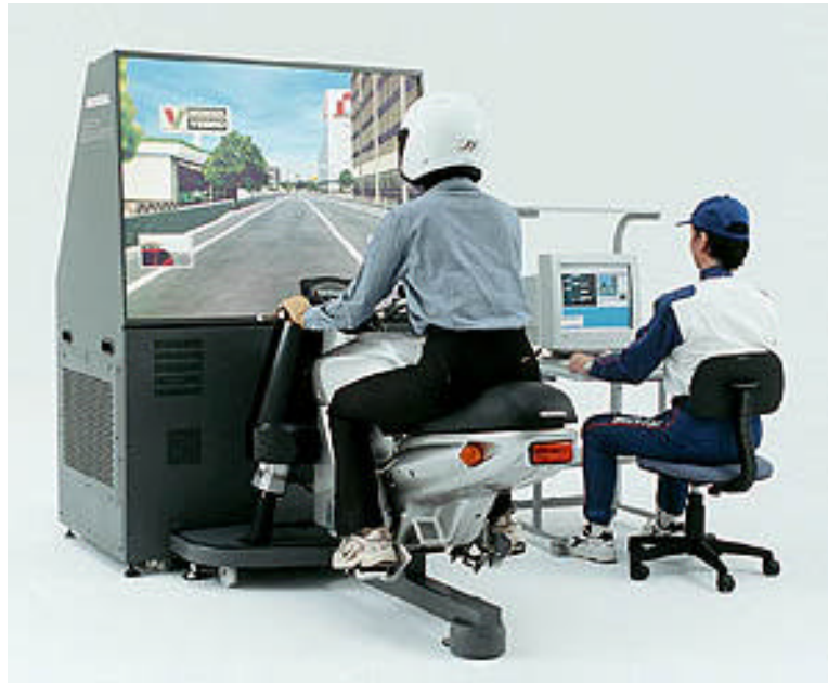
Figure 8.2 The second generation Honda motorcycle riding simulator. Image from http://world.honda.com/news/2001/c010417_1.html
