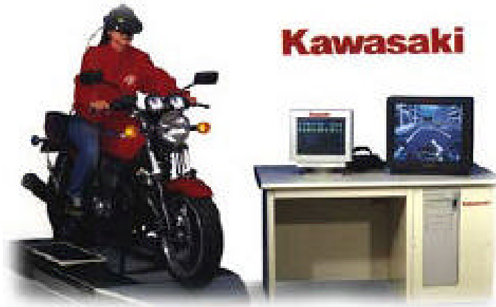
Figure 8.3 The Kawasaki motorcycle simulator incorporating a head mounted display. Image from www.phrixus.com/training.htm
