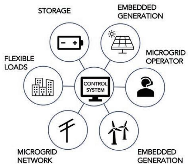
Figure 1 // Components of a Precinct Microgrid
