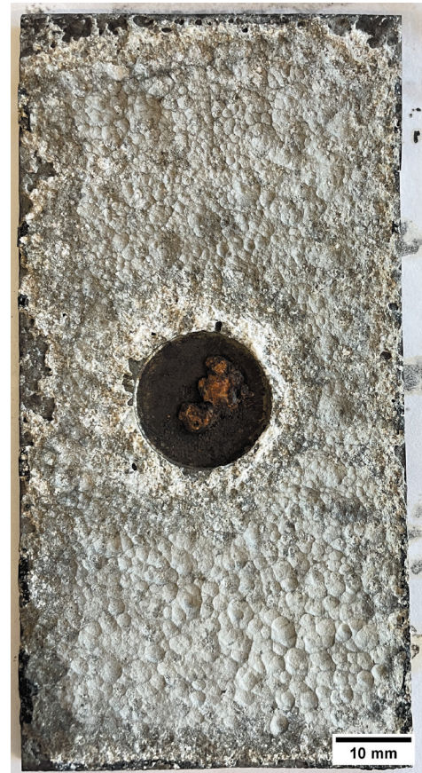
Cold spray aluminium coating after exposure to salt spray test at 60°C
