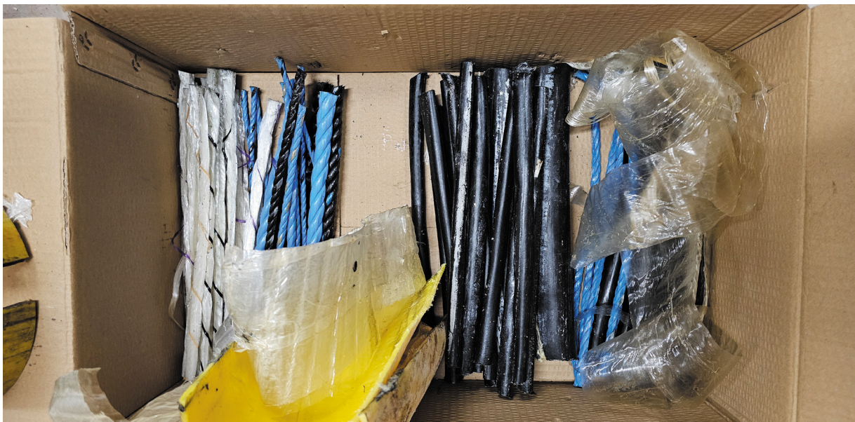
Deconstructed umbilical separated into polymer classes to explore recycling pathways
