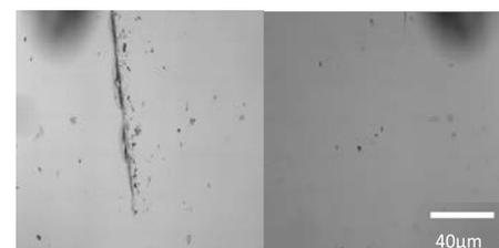
*Figure 1:* Optical micrograph of scratched (left) and healed coatings (right) formed by co-polymerising our photo-degradable dimer with (A) hexyl methacrylate monomer and (B) ethyl acrylate monomer.
