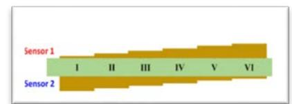
Figure 1. Nanowires grown on a substrate with sequential regions masked.
