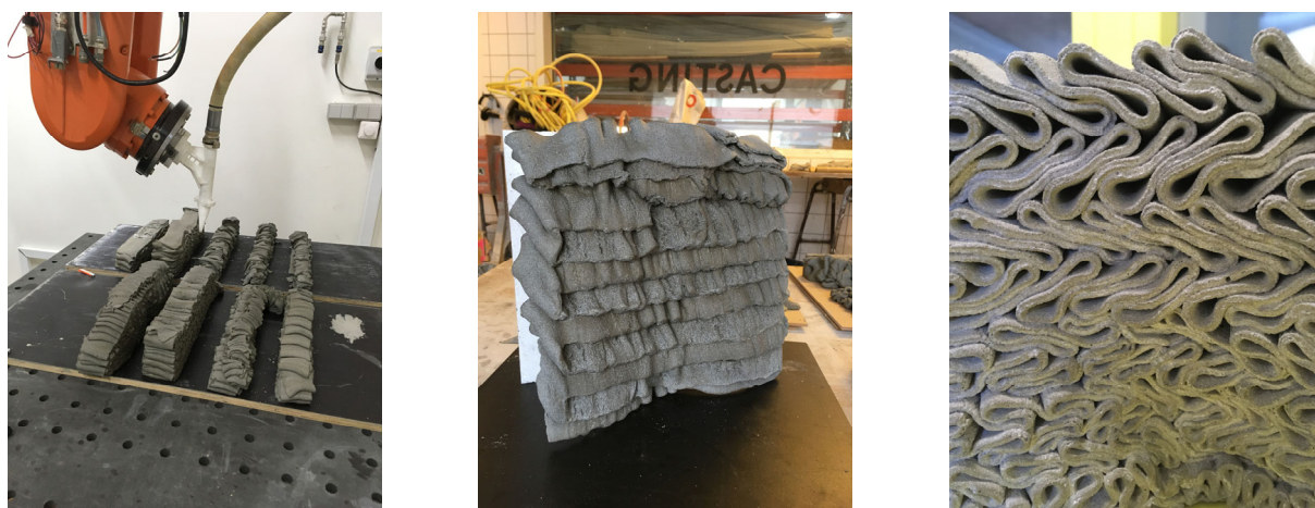
Figure 19. Initial concrete 3D printing test, both by robot and by hand
