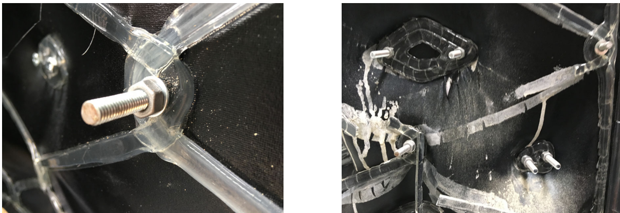
Figure 9. PLA clamping detail before casting and collapsed print after the pour.
