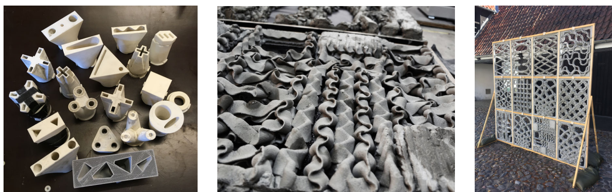
Figure 20. End-effector nozzles, detail from a printed panel and wall assembly.
