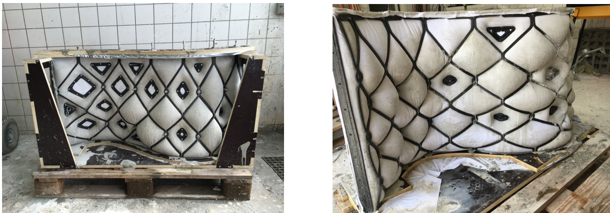
Figure 11. Concrete casts in formwork printed with the redesigned thermoplastic hybrid.
