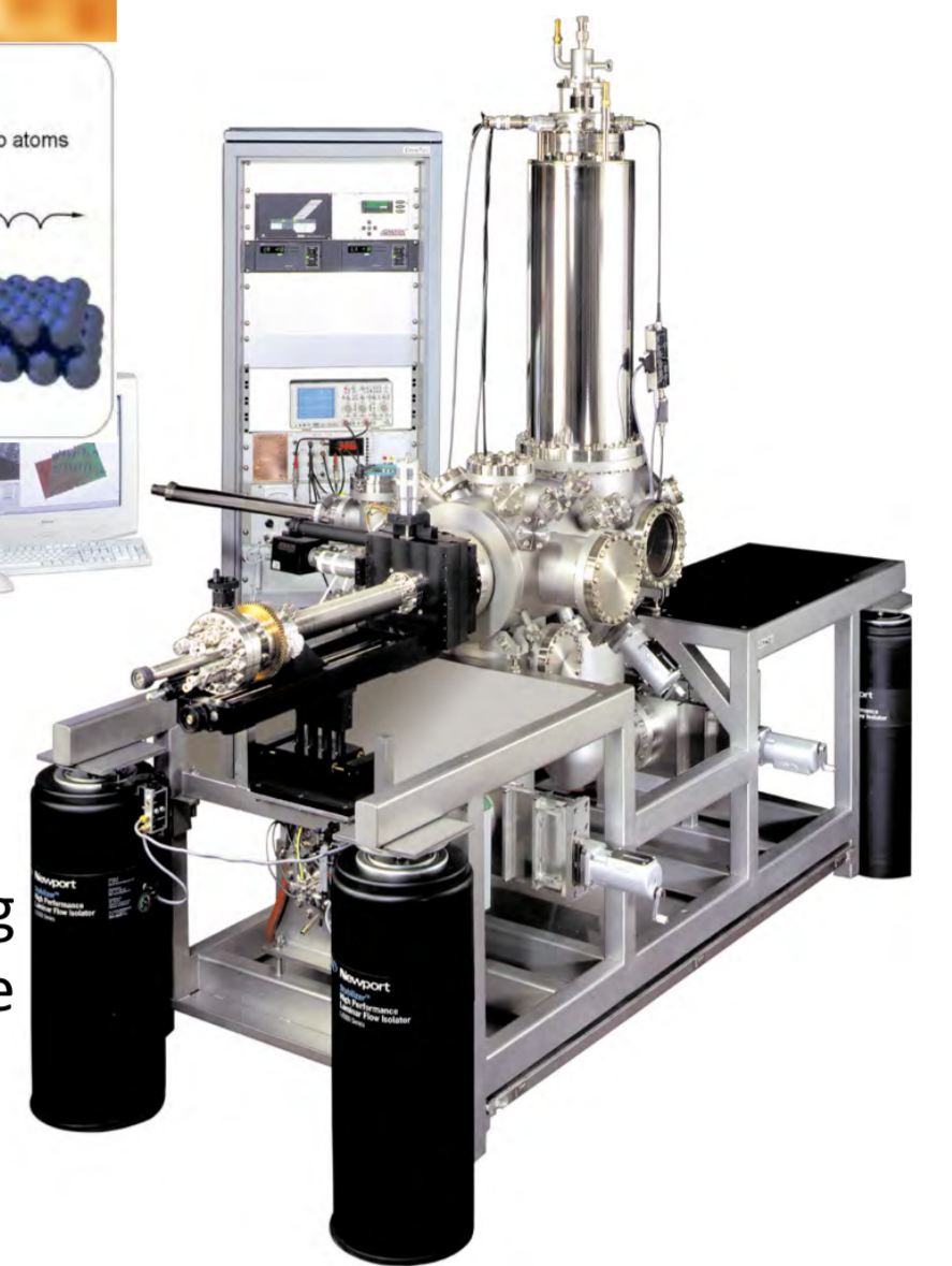
Low-temperature scanning tunneling microscopy of Na 3 Bi grown by molecular beam epitaxy
