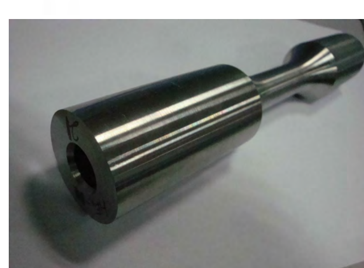
Specimen type 2: Thin-walled tubular specimens (ASTM E2207-02)
