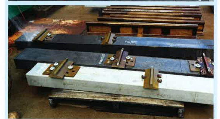
BOTH IMAGES: Electrical testing assembly. Institute of Railway Technology
