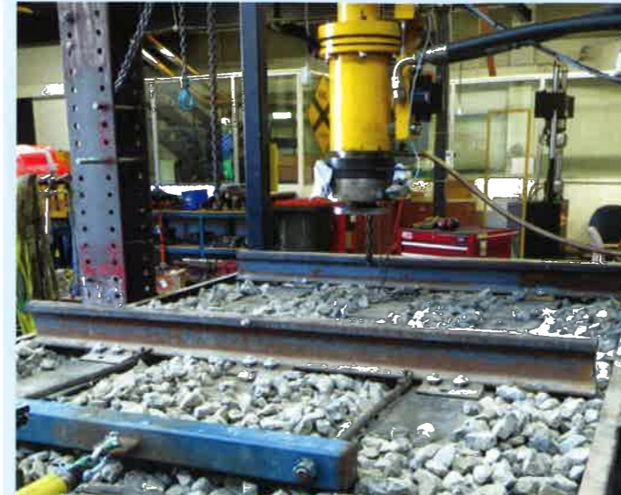
Sleeper Lateral Stability Test assembly. Institute of Railway Technology
