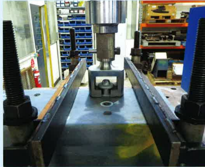
An example of the pull-out test. Institute of Railway Technology
