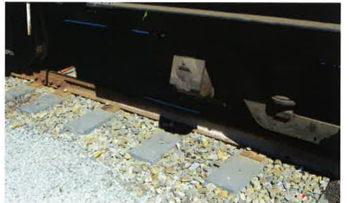
Sleeper Lateral Stability Test assembly. Institute of Railway Technology
