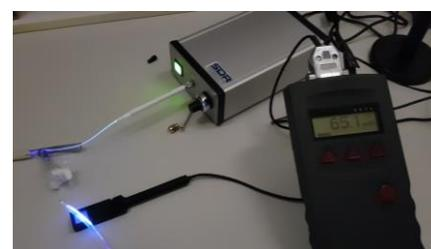
**Figure 1.** Light source connected to the Lumi-Solve device, along with a device for measuring the intensity of light emitted.
