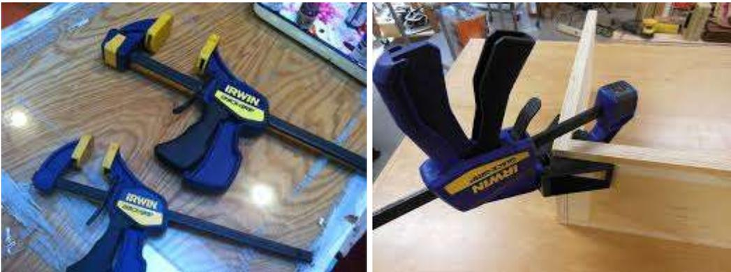
Quickgrips are extremely versatile and easy to use to hold your workpiece to a bench or hold multiple pieces of material together. Ideal for assembly of projects and holding material while you use a cordless drill to drill holes, etc. The soft jaws won't mark or damage most timber.
