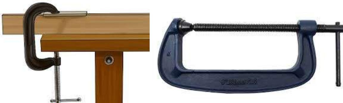
Metal G – Clamps can be used similar to quickgrips but require a little more dexterity to do up in place but can be tightened to clamp much firmer. Ideal for clamping work to be glued together or for securing work to a drill press. Be sure to use packing timber to protect your work from the metal clamp.
