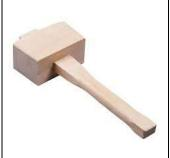
**Wooden Mallet:** used in woodwork for gently knocking timber pieces or joints together or driving in dowels. The wooden head will not damage or mark other timbers like a metal hammer. Also commonly used for hitting chisels as they will not damage the chisel handle.
