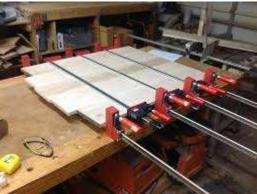
Large Bar clamps are ideal for glueing pieces of timber together to make large pieces of work such as table tops.
