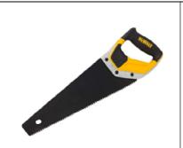
**Crosscut Saws:** are very common handsaws for manually cutting wood across the grain. Each cutting tooth is angled to cut with one edge and push sawdust out with the other. Their blades contain 8 to 15 TPI.
