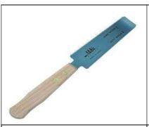
Flush Cut Saws: are double edged tools designed for trimming the ends of dowels, tenons, and other protrusions flush with the surface. The blade bends to lay flat on the flush surface and its teeth are angled upwards to prevent surface marring. The blade is about 6 inches long and usually has 11 TPI on one side and 20 TPI on the other for versatility.
