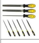
Files are ideal for removing burs and sharp edges after cutting processes or shaping metal materials and enlarging holes. They come in rectangular, round and half round styles and in numerous sizes. Coarser teeth "bastard" files remove material faster, while finer teeth "smooth" files are used for finishing.
