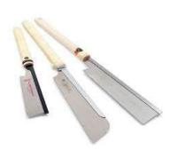
**Japanese Saws:** are an accurate type of woodworking saw that <u>cut on the pull stroke</u>. As a result the blade cuts under tension and can be thinner with a finer kerf and is more efficient. They can be rigid back saws or more flexible such as a flush cut saw.
