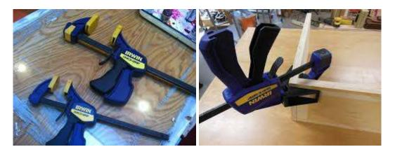
Quickgrips are extremely versatile and easy to use to hold your workpiece to a bench or hold multiple pieces of material together. Ideal for assembly of projects and holding material while you use a cordless drill to drill holes, etc. The soft jaws wont mark or damage most timber.
