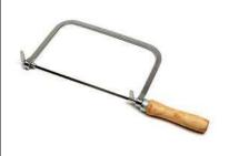
**Coping Saws:** are used to make curved cuts on thinner materials. They use a very thin metal blade with a U-shaped frame and wood or plastic handle to make turning cuts on wood, plastic, or metal depending on the selected blade. Blades usually have 12 to 15 TPI, but coarser and finer blades are available for specialized applications.
