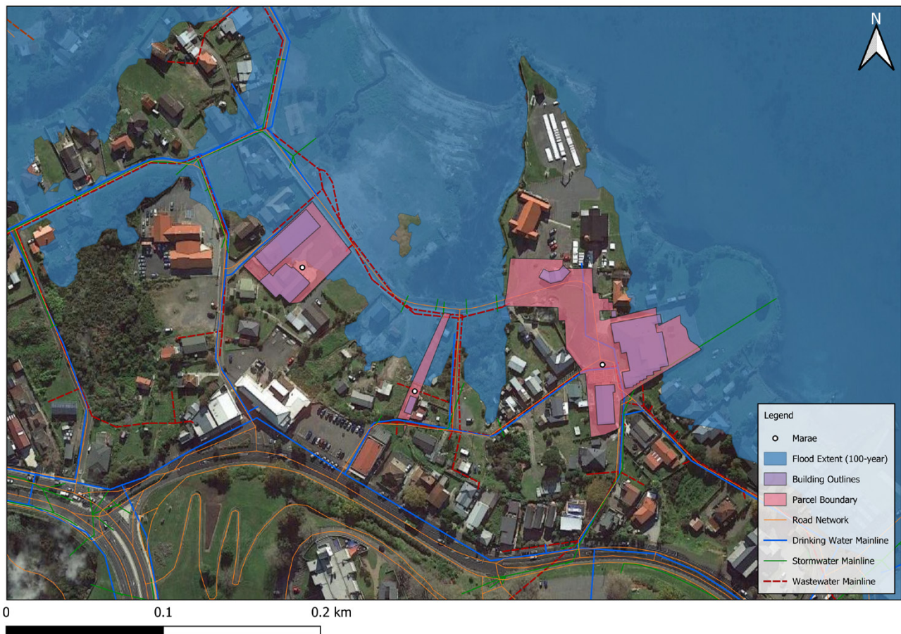
Figure 5: Marae flood map showing 3 marae in close proximity along with site boundaries, building outlines, infrastructure networks and a specific hazard.
